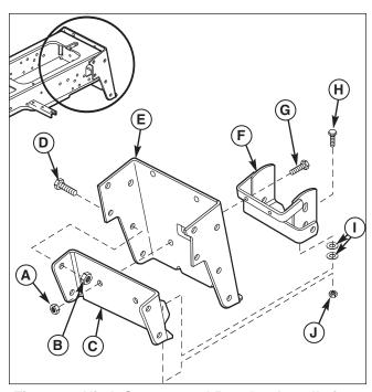
Figure 5. Hitch Support and Drawbar Installation
